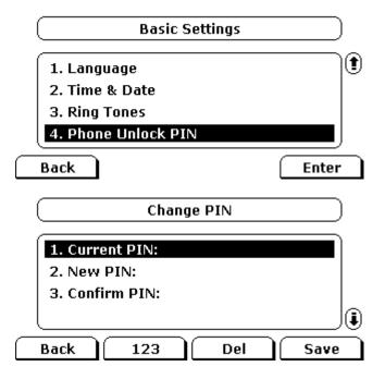
**Description :** it can be used to configure the unlock PIN on LCD. And the default value of the PIN is '123'.
